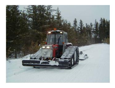
Our Unit 2 the New Holland has a newer drag installed and we have done some hydraulic updates to control the drag better. It is not a new unit but has a strong heart and is ready to roll.
